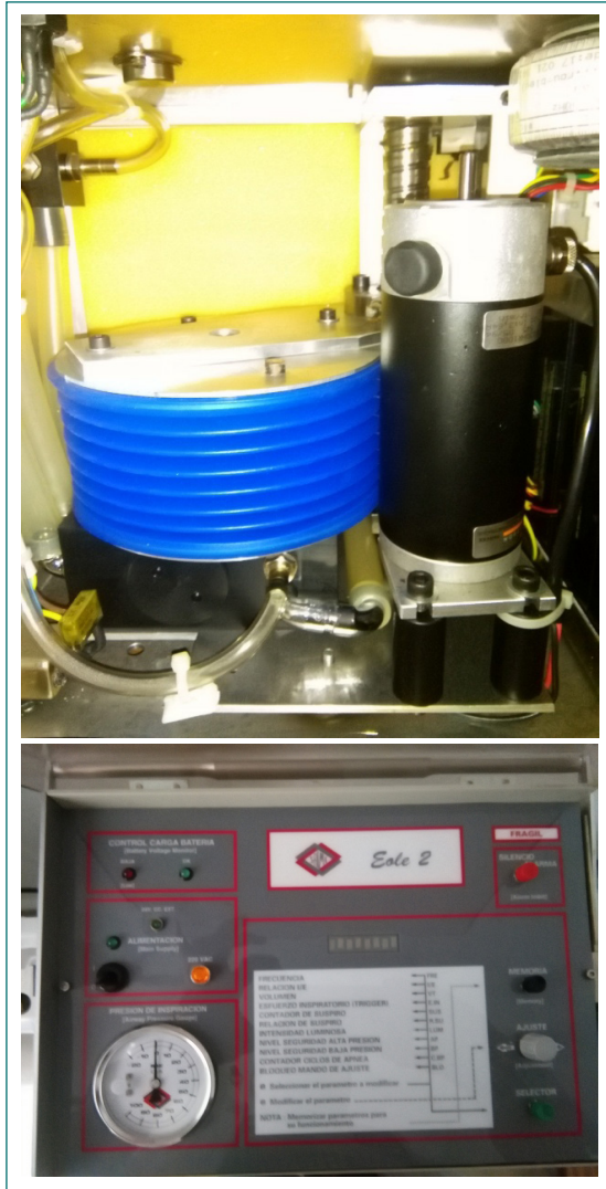
Figure 1. Volumetric ventilator (Eole 2, Saime, France) from the late 1990s/early 2000s. Note the few electronic components and the analogue pressure gauge as the sole monitoring element.
