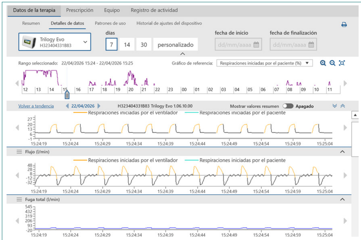
Figure 4. Dissociation between the patient's actual respiratory rate and that shown by the ventilator. This is a neuromuscular patient with no real capacity for autonomous breathing, with complete ventilator dependence. In the upper image, it can be observed that during daytime periods the patient triggers almost 100% of inspirations ("assisted" breaths), whilst at night the ventilator remains at the back-up rate (0% assisted breaths, all controlled). On detailed review of the ventilator record, it was found that with a flow trigger of 5 L/min, the effect of the cardiac beat (cardiobalistic effect) on respiratory flow was triggering the ventilator at a high rate; this was corrected by increasing the trigger sensitivity to 7 L/min ( continued ).
